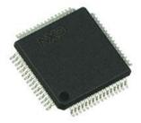
The microprocessor that has been used for this project is a 32 bit ARM7, CPU with real-Time emulation and embedded trace support that combines the microcontroller with 512 Kb of embedded high speed Flash memory. It has two 8 channel ADC, single 10 bit DAC, two 32 bit timer/counter ,multiple serial interfaces including two UART ,two fast I2C, Capture, compare and PWM module.
